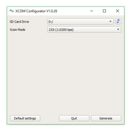
After downloading and installing the Xcom-Configurator, you are able to change the baudrate:
