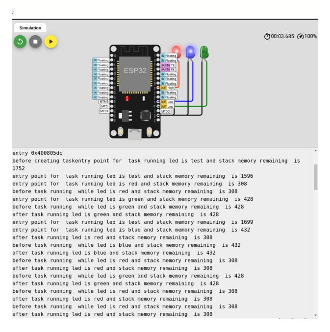
Note: Reason for different stack size when we call uxPortGetSackHighWaterMark() API function: Stack is responsible to save all variables initialized as well as execution state during "context switch", therefore, it is possible to have different stack consumption for functions having same implementation due to different states during context switching.
