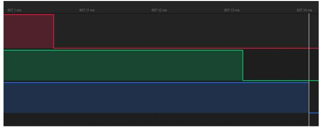
Time to start task1 : 607.105 ms Time to start task2 : 607.131 ms Time to start task3 : 607.141 ms difference Task2 - task1 = 0.026 ms Task 3 - task 2 = 0.009 ms
