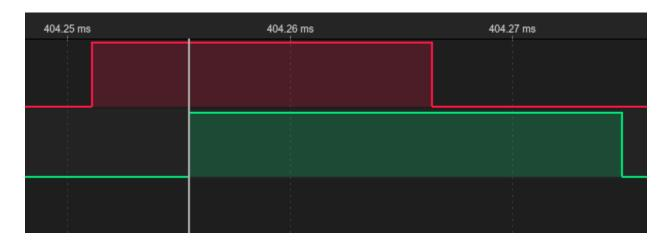
Receiver task is implemented to get 5 values only in one complete iteration , therefore, it has low execution time as it takes less time to get value from Queue as shown in previous test. In this test , as soon as value is removed from Queue, a place is empty therefore, Sender Task Preempt Receiver Task.
