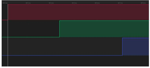
Time to start task1 : 507.212 ms Time to start task2 : 507.436 ms Time to start task3 : 507.709
