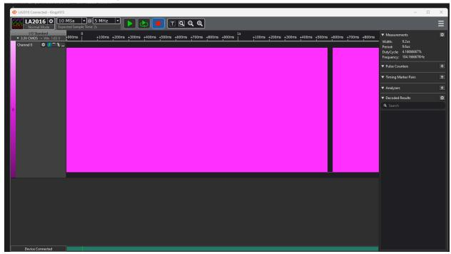
1 Task with 1 ms as delay (defualt Tick Rate is 100 Hz which means 10 ms period).
